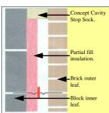
During horizontal installation it is advisable to protect the Cavity Stop Sock with a damp proof course or proprietary cavity tray immediately above with a minimum 100mm upstand.
