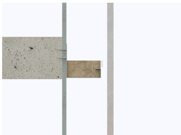
Side view showing rainscreen barrier held in place by the unique retaining bracket
