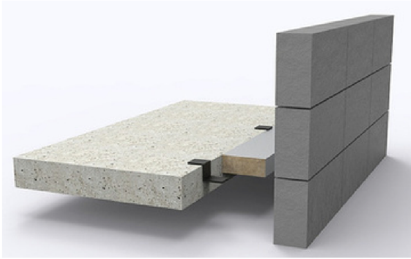
Horizontal Firestop between floor slab
